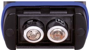
Batteries type must be of **Energizer L91** (1.5V/LiFeS technology).
