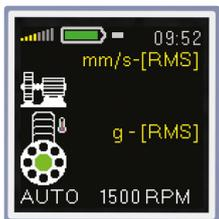
Detected speed value is displayed at the bottom. The word **AUTO** in front of the value informs, that automatic detection was used.
