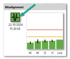
If the measured value is above the 'danger' limit, you can see that icon is red. It is dangerous fault on the machine.
