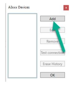
This window is blank (without any online unit added) when you start to use Omega application. You need to add your online unit with 'Add' button. Fill in units name and its IP address. You can set used sensors here. Or you can also use sensor settings from DDS – 'Read DDS sensor settings from the device'. Confirm with 'OK' button.
