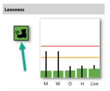
If the measured value is above the limit, you can see that icon is red. It is dangerous fault on the machine.
