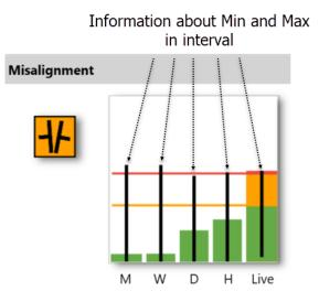
Live ... Last measured value is shown. It is refreshed every 1s. What about the line in the column? It shows Min and Max for values measured in the current 'open' hour. Min and Max are minimum and maximum value in interval 15:00 to 15:30.
