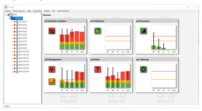
OMEGA engine itself exposes fault severity data (machine condition, unbalance, etc.) on OPC server. From OPC you can read the data by third party software and display them in the software which you already have.
